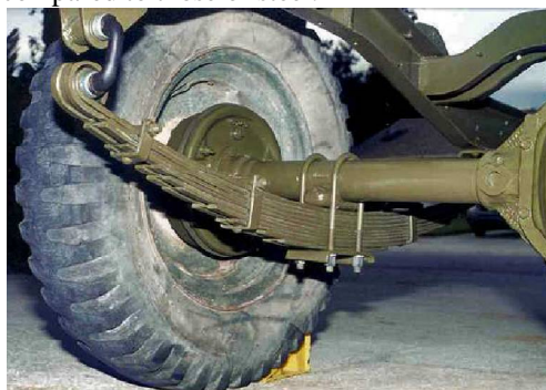
Fig.1 Leaf spring assembled at rear axle of automotive
