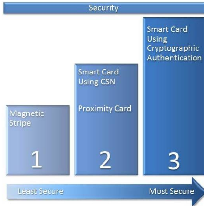
Figure 1: Relative Security Levels of Commonly Used Card Technologies (lowest to highest)[3]
