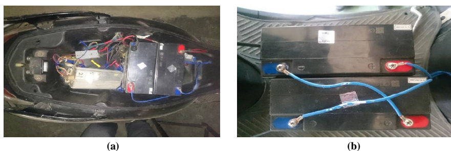
Fig. 4: Battery position in hybrid two-wheeler prototype, (a) Batteries in boot & (b) Batteries on foot space
