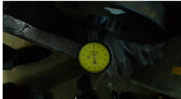
b) Run-out Measurement
