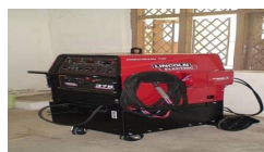
Fig.1. TIG welding machine
