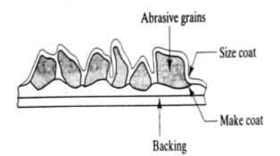
Abrasive belt grinding is a common finishing process in the metal and wood working industries. Coated abrasive belts are used in the same speed range as bonded wheels, but they are not generally dressed when the abrasive becomes dull. The wide spread application of coated abrasive belts and long standing operating practices have led to different kinds of quality requirements. The abrasive belt machining technique is more significant for precision machining and finishing.
