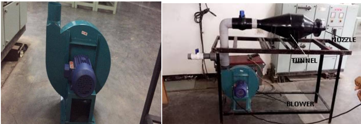
Fig 3.1.4 (a) Blower (b) Final Assembly
