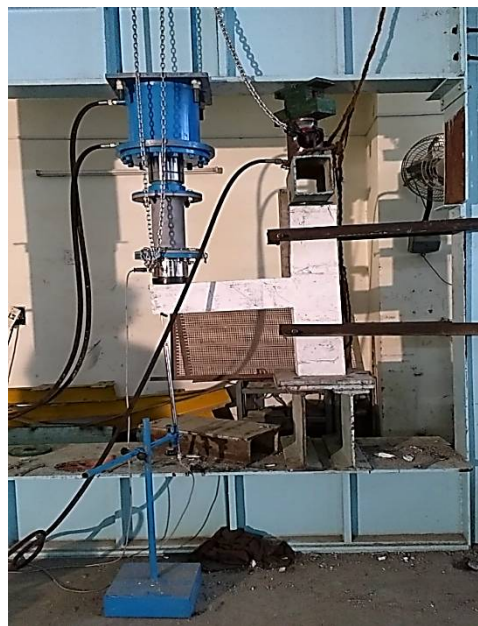
Fig 3: Testing of Beam-column joint
