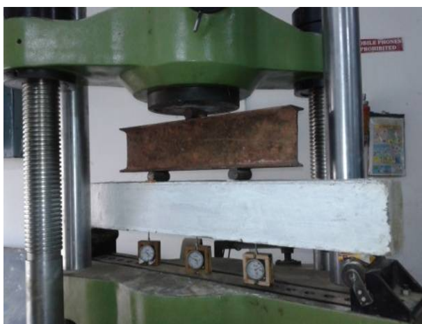
Figure 2: Beam Under Loading Condition
