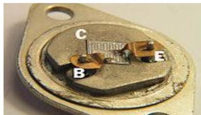
Fig: 5 Internal parts of transistor 2N3055
