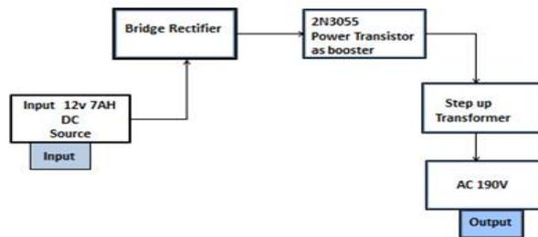
Fig:2 Block diagram of boosting and conversion of power
