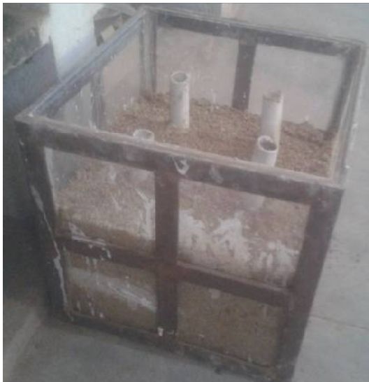
Fig 3.1: lime grouted tank
