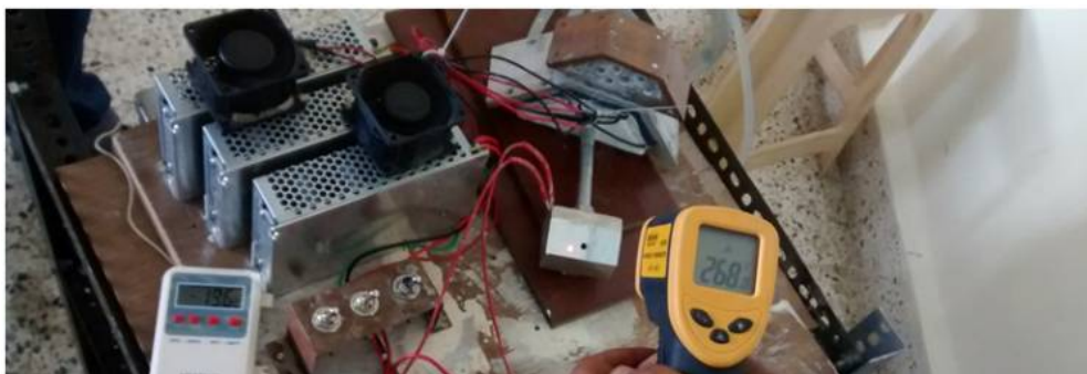
Fig. 15 Simultaneous operation of Desorptor and Condenser. (@-19.6°C & +268°C)
