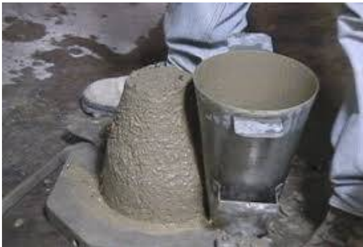
Slump Cone Test
