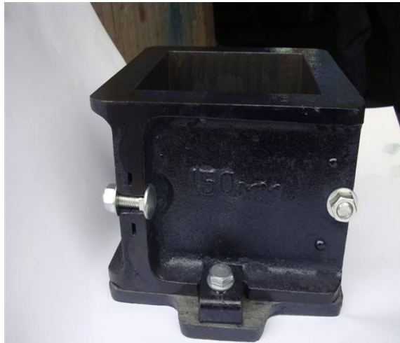
Casting of concrete cubes
