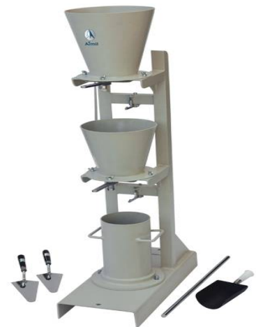
Compaction Factor Test
