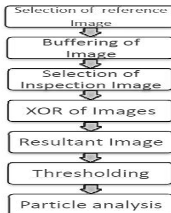
Fig. 3 Inspection flow chart-
