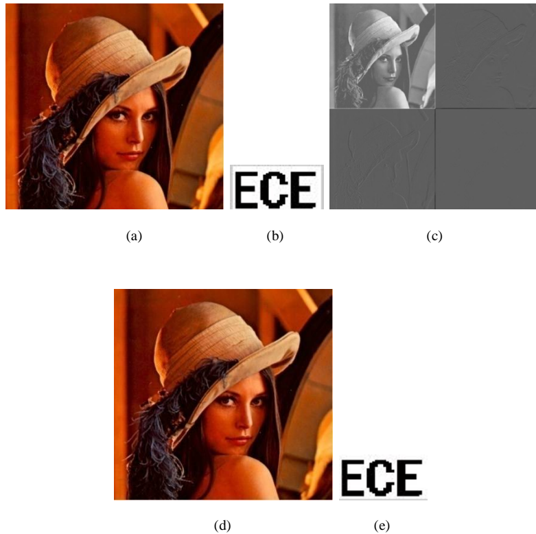
Fig. 6. Digital Image Watermarking (a) Original host image of size 512X512 (b) Binary watermark image of size 32X64 (c) DWT host image(Haar wavelet) of size 512X512 (d) Watermarked image of size 512X512 (PSNR=48.16dB) (e) Extracted watermark of size 32X64 (NCC=1)
