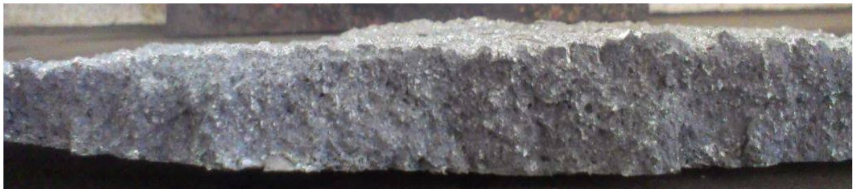
Figure 1 Spray formed Deposit-Side view
