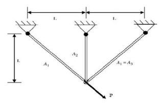
Fig.1. Design of Three Bar Planer Truss
