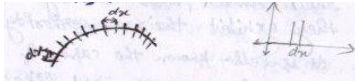
fig.1:-Arrangement of parts to make circular like arrangement of bricks to make circular path / wall.
