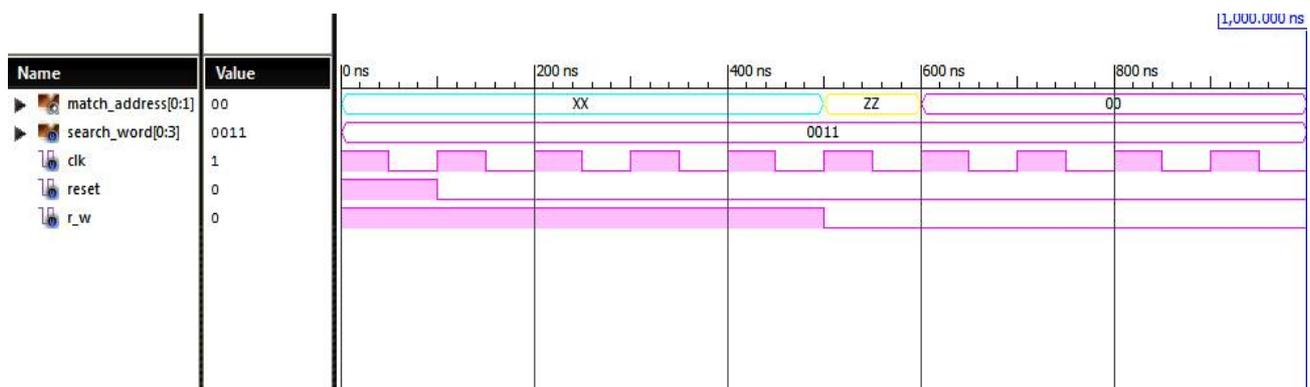
Fig. 7: output waveform of modified Z-TCAM
