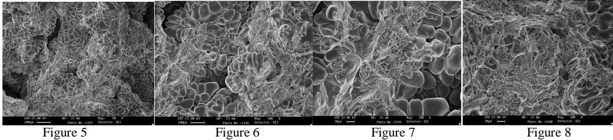
Figure 5 to Figure 8 shows the SEM micrograph of MMC of Al with 6% fly ash at different resolutions. Figure 5 shows the micrograph of MMC of Al with 6% fly ash at 50X magnification. Figure 2 shows the micrograph of MMC of Al with 6% fly ash at 100X magnification. Figure 3 and Figure 4 shows the micrograph of MMC of Al with 6% fly ash at 200X magnification. By these micrographs we see that the fly ash is mixed with aluminium and give us better properties than aluminium.
