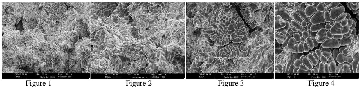
Figure 1 to Figure 4 shows the SEM micrograph of pure Al at different resolutions. Figure 1 shows the micrograph of pure Al at 50X magnification. Figure 2 and Figure 3 shows the micrograph of pure Al at 100X magnification. Figure 4 shows the micrograph of pure Al at 200X magnification. These micrographs are used as reference which is used to compare the micrographs of MMC.
