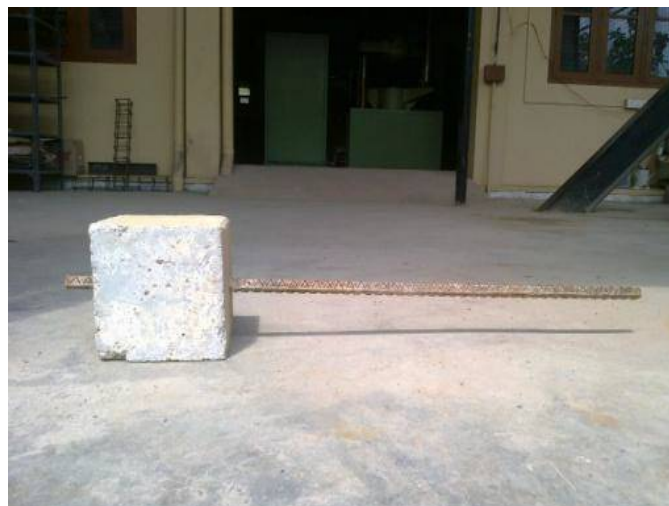
Fig. 1. Pullout Test Specimen
