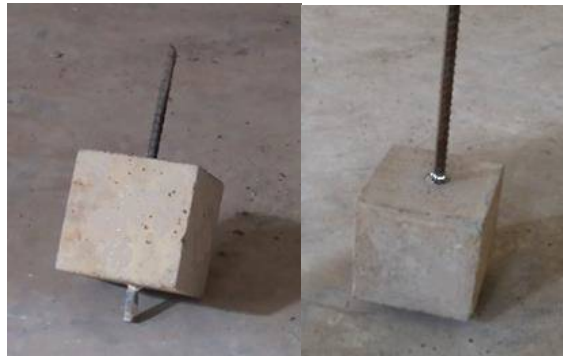
Fig 3. (a)Yield Failure. (b) Pullout Failure
