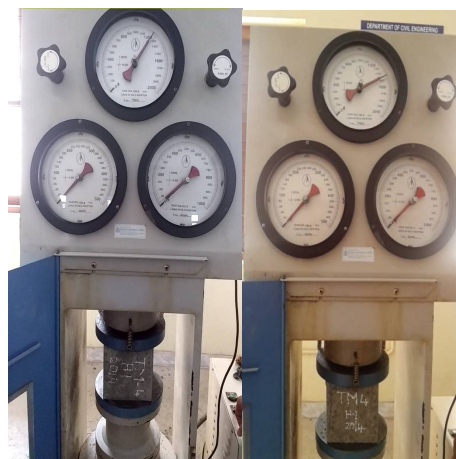
Fig 4: Setup of compressive test for trial mix 4
