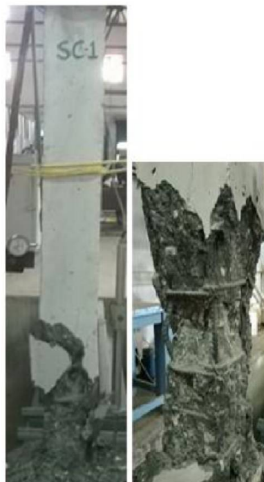
Fig. 4. Failure patterns of square control specimen
