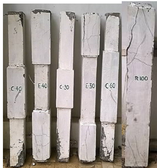
Fig. 6. Failure patterns of partially jacketed and rehabilitated specimens
