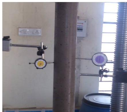
Figure 5. Extensometer connected over concrete column
