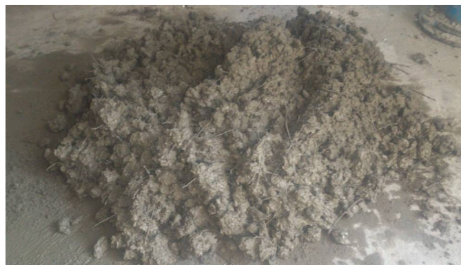
Figure 3. Concrete mixed with steel fibres
