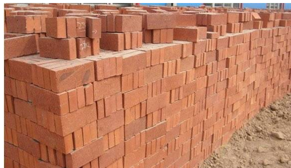
Fig. 3. Burnt clay bricks
