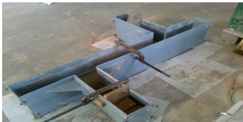
Fig. 6 Steel Frame Used For Casting of Beams
