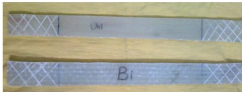
Fig.7 Uni-GFRP & Bi-GFRP Specimens for testing
