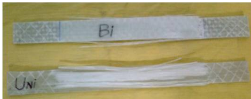
Fig.8 Failure of Uni-GFRP & Bi-GFRP Specimens after tensile test
