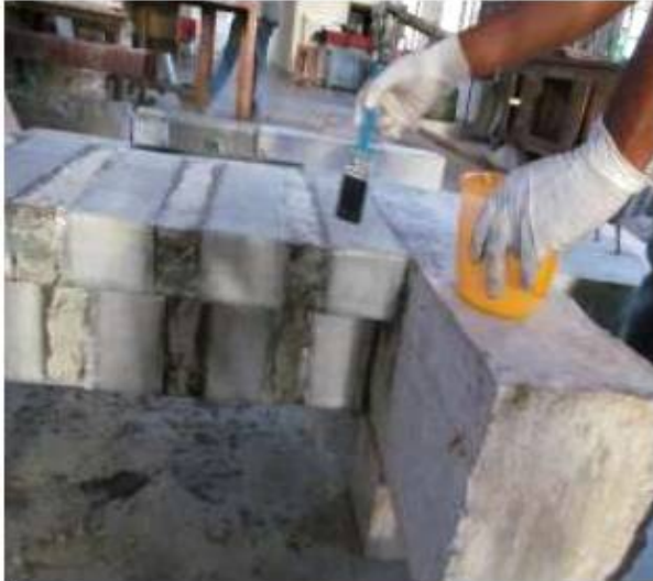
Fig. 1 Application of epoxy and hardener on the beam
