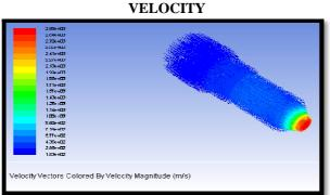
According to the above contour plot, the maximum velocity is 2.96e+03m/s and minimum velocity is 1.53e+02m/s.
