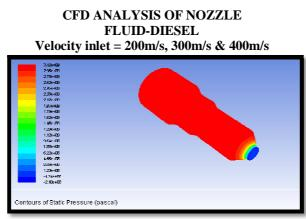
According to the above contour plot, the maximum pressure is 3.12e+09Pa and minimum static pressure is -2.10e+08Pa.
