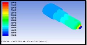
According to the above contour plot, the maximum heat transfer coefficient is  $3.59e+05w/m^2-k$  and minimum heat transfer coefficient is  $1.80e+04w/m^2-k$ .
