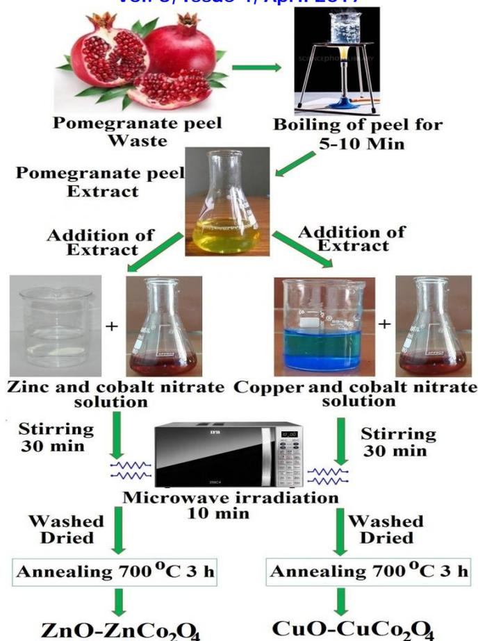
Scheme.1: Step wise synthesis procedure for the composites.
