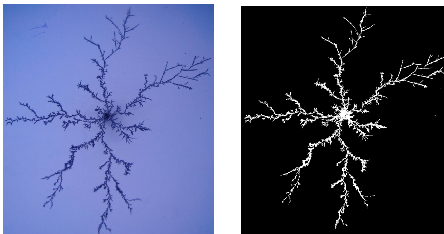
Fig. 2 Electrodeposit form 1M zinc acetate solution at cell voltage of 5 V and the same image after converting to two colour bitmap.
