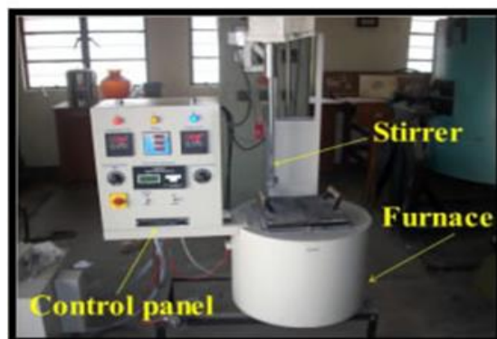
Fig 2.2: Components stir casting process
