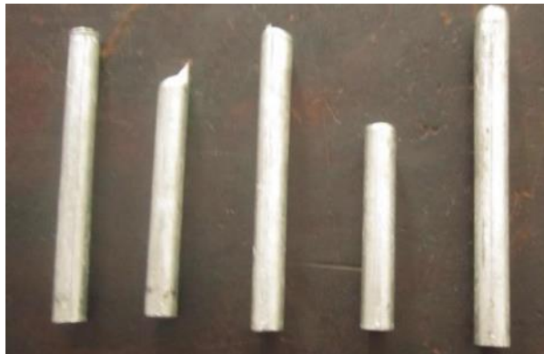
Figure 2.3.1 Different weight fractions of TiB_2 reinforced MMC's
