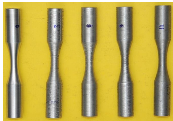
Figure 2.3.2 Machined ASTM Fatigue test specimens for different weight fractions of TiB_2
