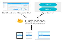
An FCM implementation includes an app server that interacts with FCM via HTTP or XMPP protocol, and a client app. You can compose and send messages using the app server or the notification console.
