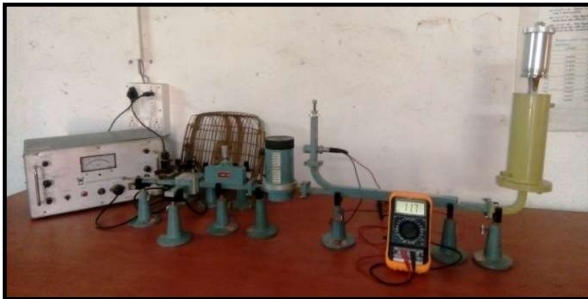
Figure 1. X-Band Microwave Technique Experimental Setup with Liquid Dielectric Cell.
