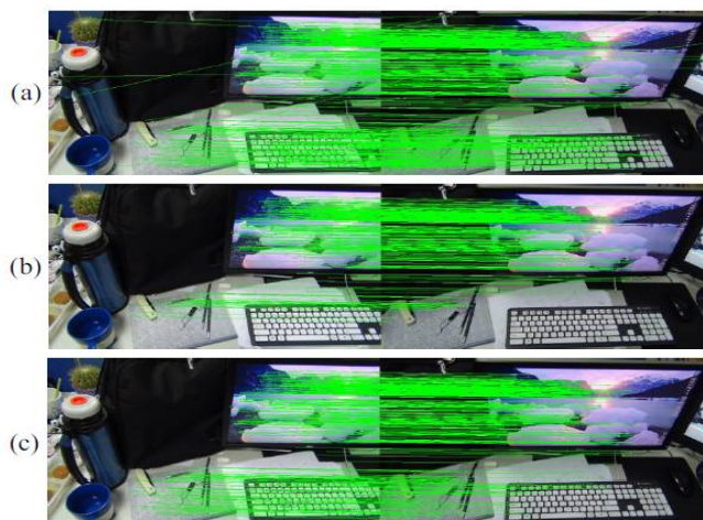
Fig. 2: Outliers rejection comparison. (a) Matched features by SIFT. (b) Recognized inliers by RANSAC with global homography. (c) Recognized inliers by our approach.
