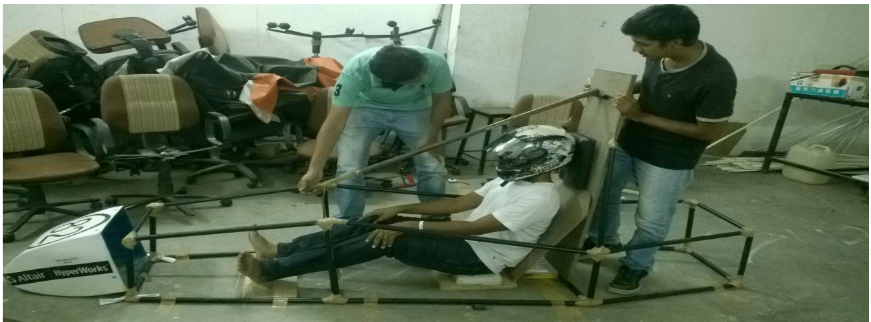
Fig 7:- Driver seating position in the prototype made up of PVC pipes
