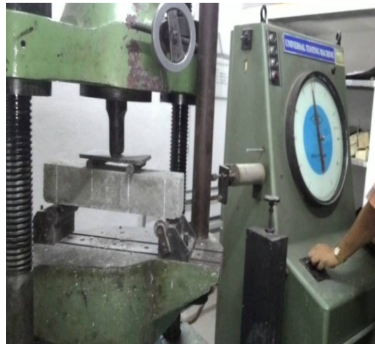
Photo.2 Testing of prisms
