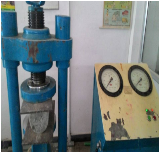
Photo .1 Testing of cylinders
