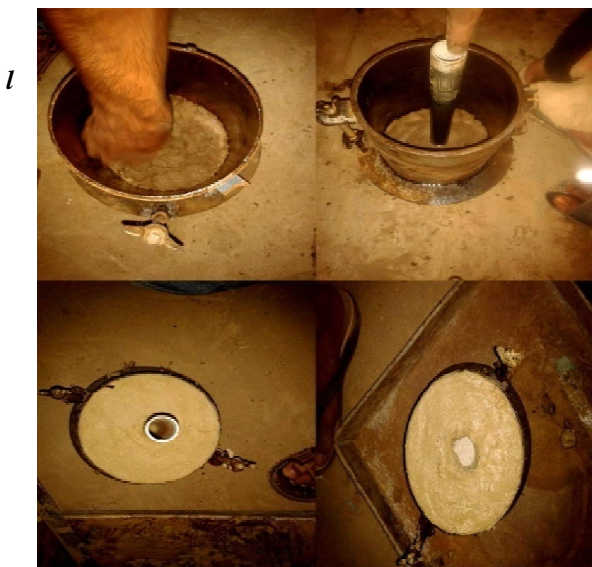
Fig:1 Installation of stone columns
