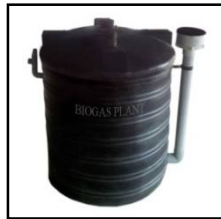
Figure 2(d): Photograph of DOMESTIC SCALE BIOGAS PLANT (1000L) that was constructed and used in the present work.
