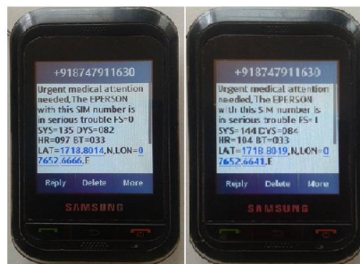
Fig. 9. Cell phone with SMS sent by developed system
