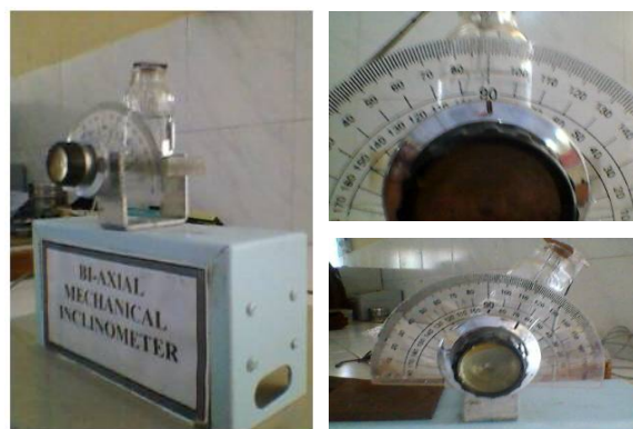
Fig. 6. Shows bi-axial mechanical inclinometer for fall angle measurement & right image shows 24 deg fall angle
