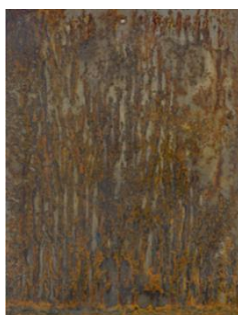
Figure 3: Typical sample after 5 cycles of alternate immersion
