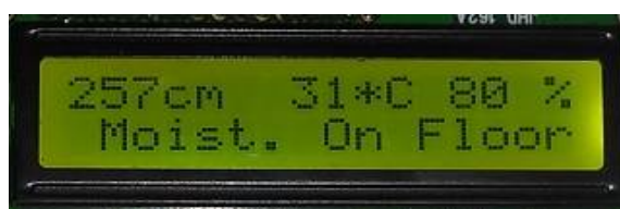
Fig 7: Moisture is detected
