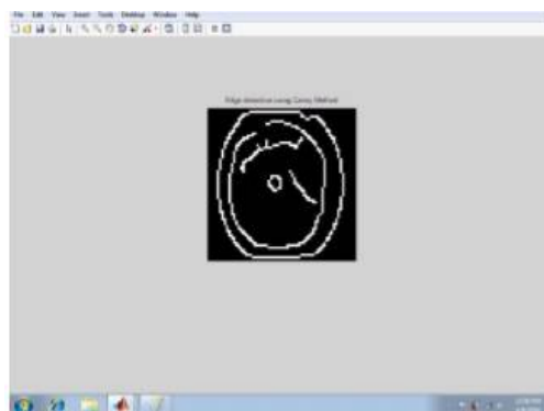
Fig 6: edge detection using Canny method
