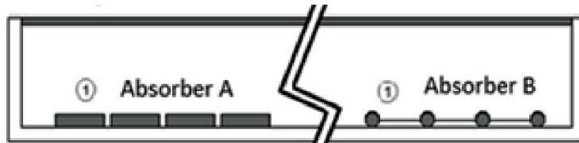
Fig.7 Circular and Rectangular absorber tube
