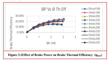
From fig 3.1, Brake thermal efficiency increases with increase an engine loads with rated speed. From the graph it is concluded that the maximum Brake thermal efficiency is obtained for 24.52% at 11.9 kg load at 180 bar pressure with 3hole nozzle. The Brake thermal efficiency at 220 bar pressure 3hole nozzle and 200 bar pressure with 3hole nozzle is higher than 22.80% diesel 180 bar pressure.
