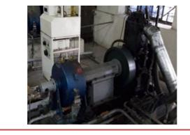
Figure 2.2. Test EnginewithDynamometer
