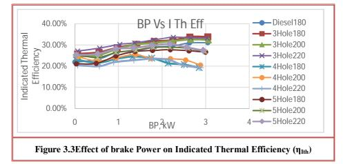
From fig 3.3, Indicated thermal efficiency increases with increase in brake power. From the graph it is observed that the maximum Indicated thermal efficiency obtained for biodiesel is 33.84% at 180 bar pressure with 3hole nozzle. The Indicated thermal efficiency value at 220 bar pressure with 3hole nozzle and 200 bar pressure with 3hole nozzle is higher than diesel 180 bar pressure.
