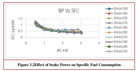
Specific fuel consumption is varies with different loading conditions and different injection pressures as shown in fig 3.2. The Specific fuel consumption obtained for diesel is 0.35 kg/kwh and 0.37 kg/kwh for animal tallow biodiesel at 180 bar using 3hole nozzle. The value is slightly difference between diesel fuel than that of animal tallow
