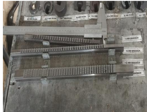
Fig.2.3 Equipment's used to produce keyway
