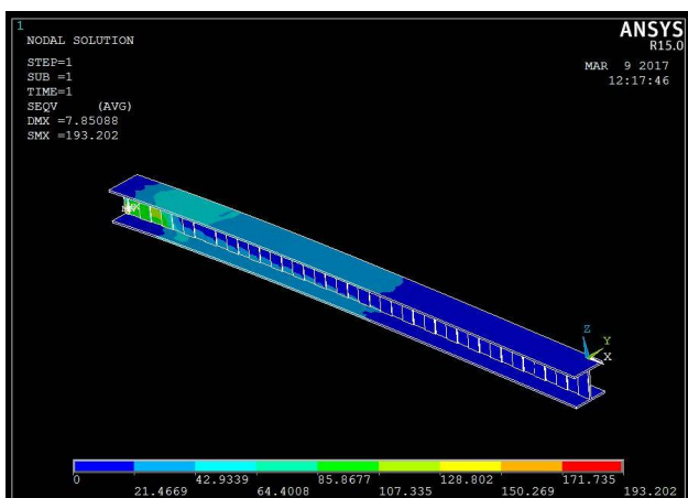
Figure 8: Von-mises stress for Boom
