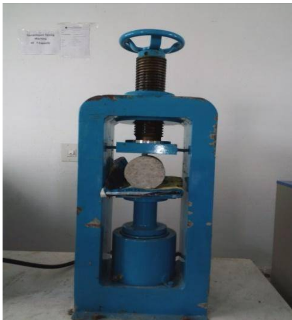
Figure 2: Split Tensile Test on Cylinders
