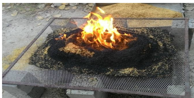
Fig. 1: Setup for burning Rice husk
