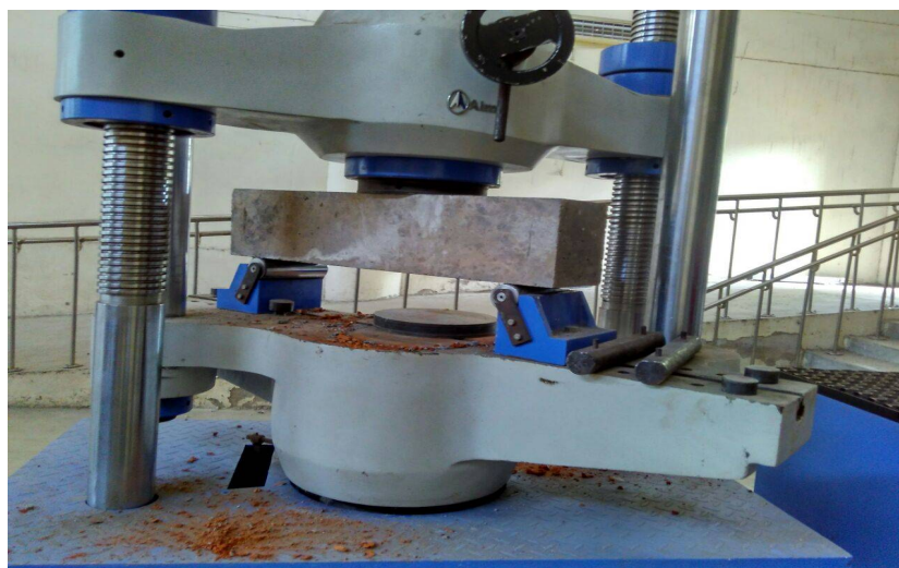
Fig. 8: Three point load test using UTM
