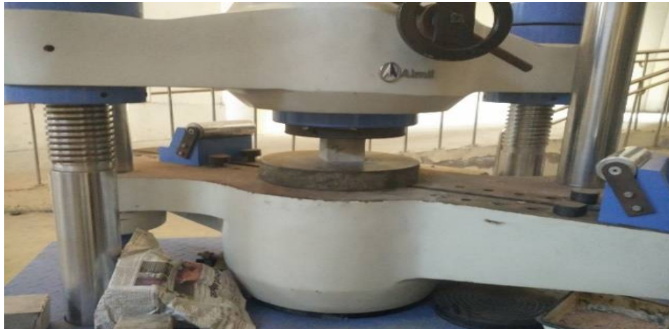
Fig. 3: Mortar test specimen under UTM
