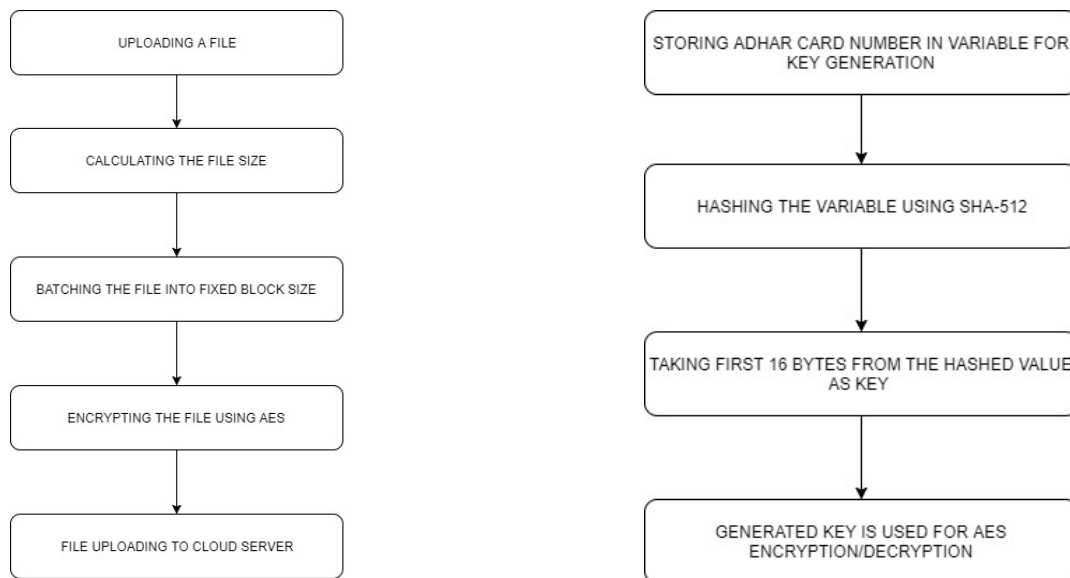
Figure 2: Steps in Uploading a File & Key Management
