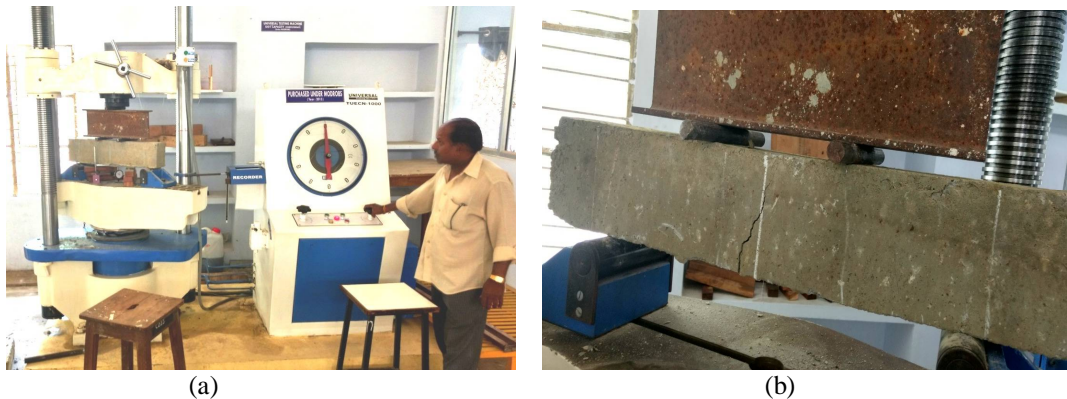
Fig. 3 (a) days cured and dried specimen arranged for flexural test (two point load) (b) Applying load in small increments, initial crack is observed and corresponding dial gauge reading is measured at mid span.
