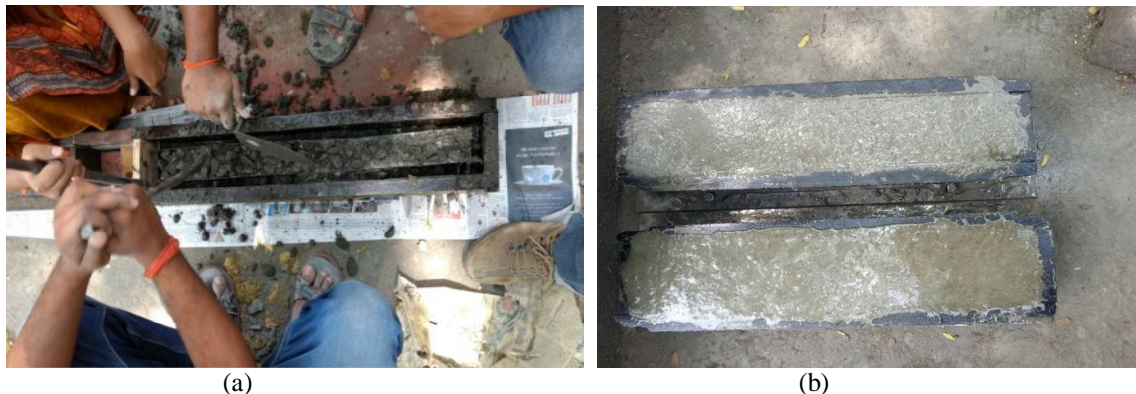
Fig. 2 (a) casting of test specimens with 20 mm cover on all the sides, (b) Finished test specimens with 20 mm cover on all the sides
