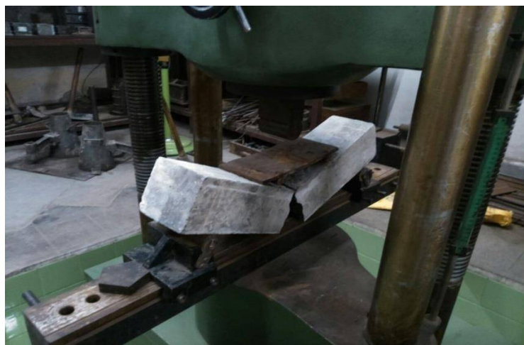
Figure 3. Testing of beam in universal testing machine
